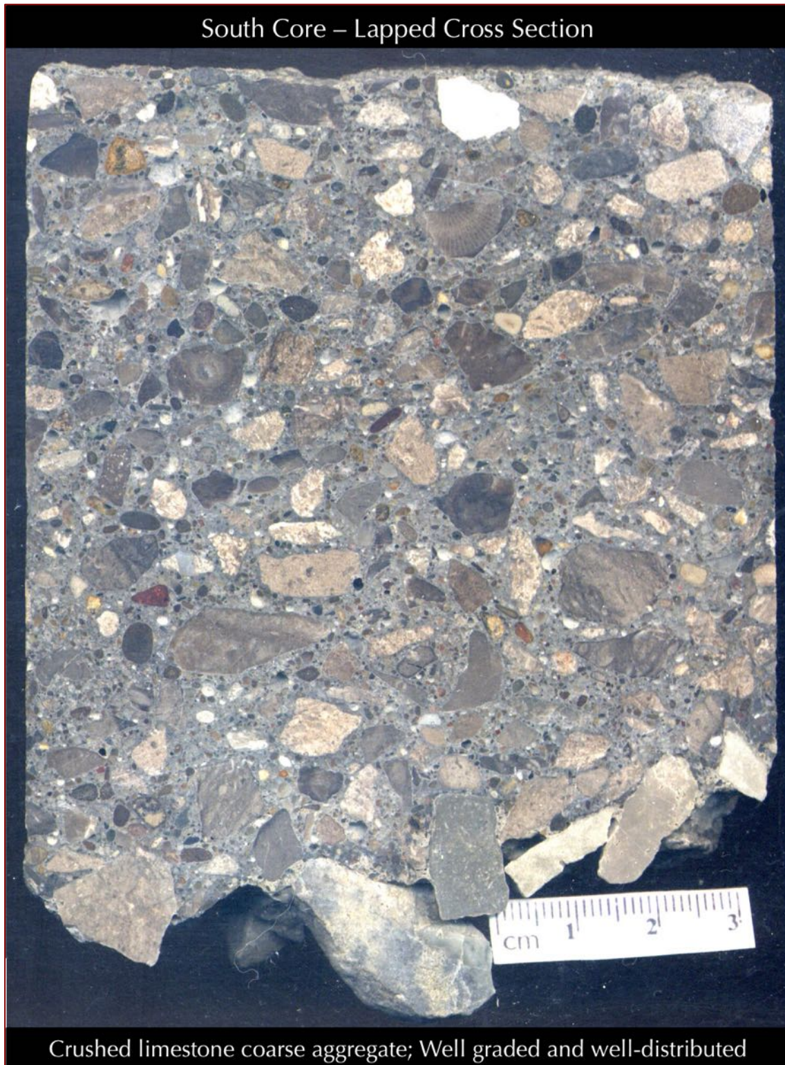
Figure 7: Lapped cross section of South Core showing: (a) severely scaled exposed surface at the top, (b) well-graded, well-distributed crushed limestone coarse aggregate, (c) dense and well-consolidated nature of concrete, (d) uniform color tone of paste in the body, but some lighter color paste at the scaled surface region at the top; and (e) adhered crushed limestone of subbase at the bottom of core.
