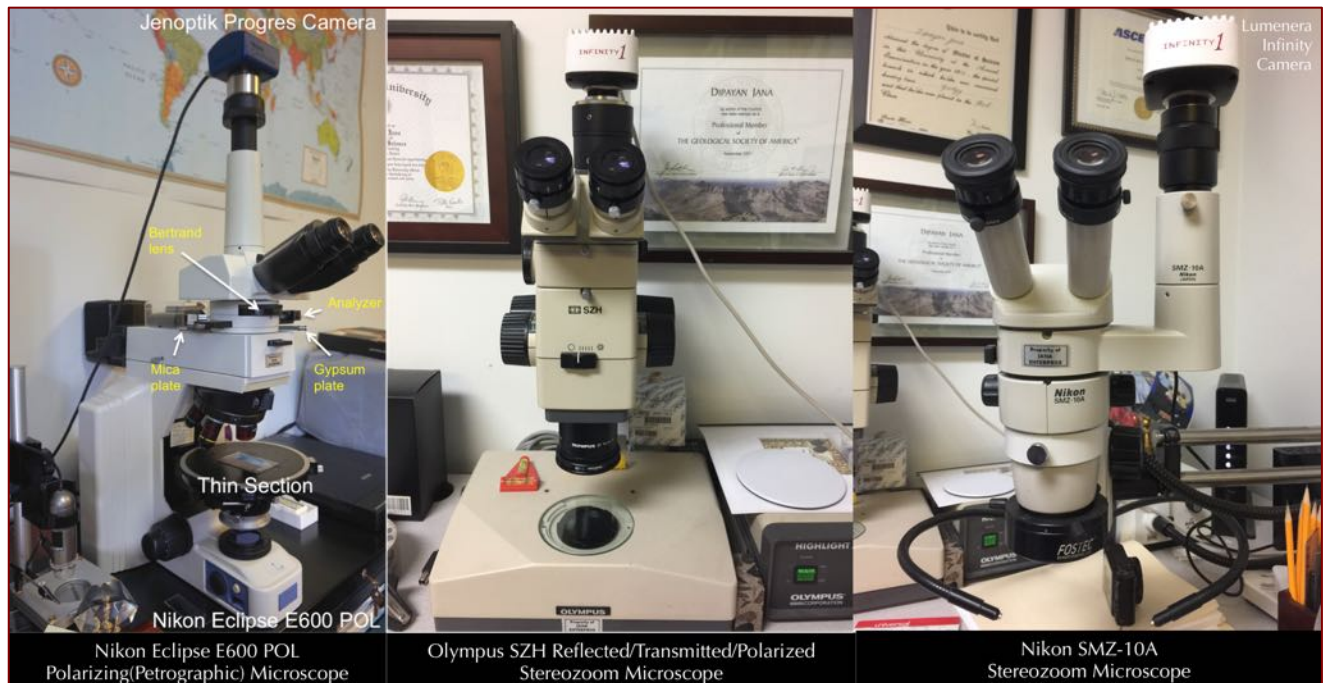
Figure 4: Nikon Eclipse E600POL Petrographic Microscope with Jenoptik Gryphax Camera (left), Olympus SZH (middle), and Nikon SMZ-10A Stereomicroscope (right) used for petrographic examinations.
