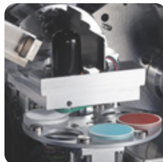
Six position sample changer
