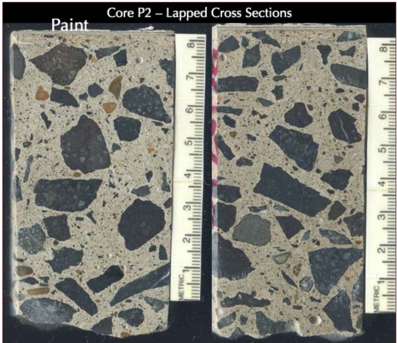
Figure 7: Two parallel lapped cross sections of Core P-2 from East Wall showing: (a) a thin paint coat at the top well-bonded to concrete; (b) no repair coat mortar topping found in the Core P- 1 from West; (c) good grading and well-distribution of the crushed stone coarse aggregate which is very different from the crushed gravel coarse aggregate found in Core P-1 from West, and siliceous sand fine aggregate particles; and (d) the overall sound, dense, well-consolidated nature of the concrete in the body of the core.
