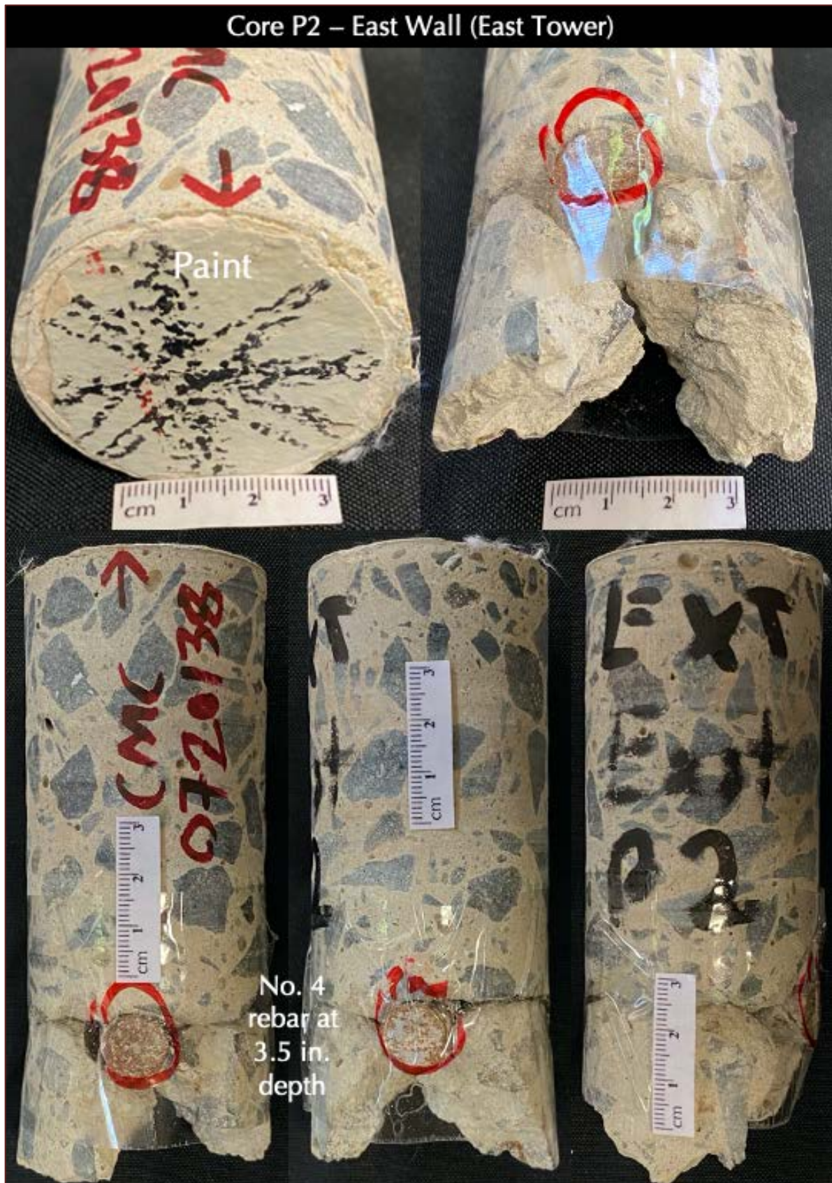
Figure 5: Shown are the exterior painted surface (top left), interior fractured end (top right) and side cylindrical surfaces of the Core P-2 from East Wall.
