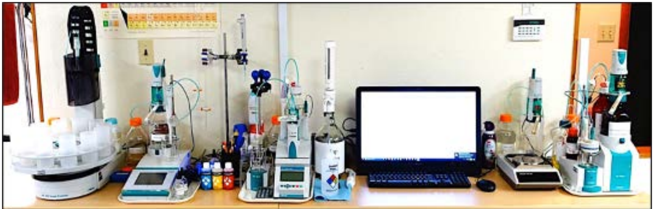
Figure 3: Set-ups for fully automated chloride analysis of concrete by potentiometric titration.
