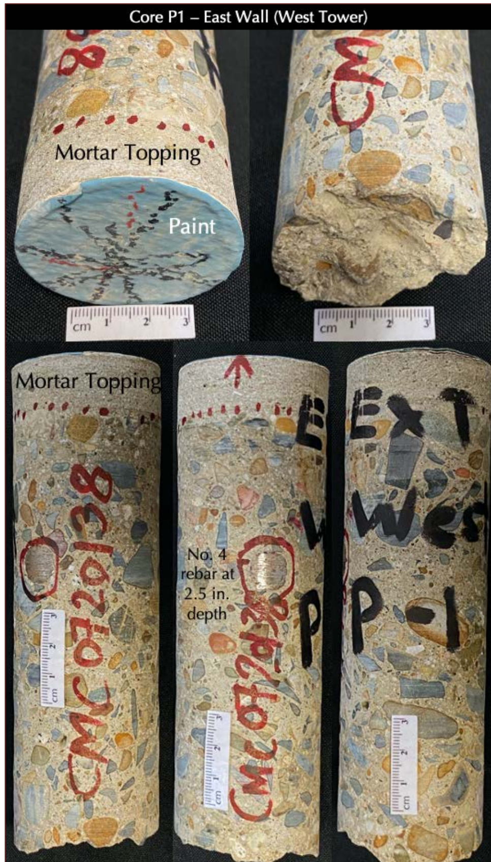
Figure 4: Shown are the exterior painted surface (top left), interior fractured end (top right) and side cylindrical surfaces of the Core P-1 from West Wall.
